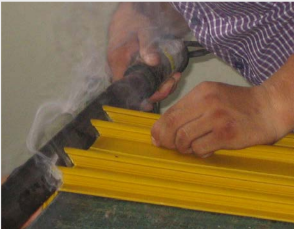
High risk of uncontrolled and improper welding due to no temperature control
